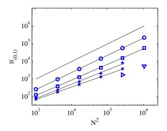
Figure 4: Effect of grid size N on asymptotic convergence rate of various optimized SRJ schemes  $(P = 2 : (\circ); P = 3 : (\Box), P = 4 : (+) \text{ and } P = 5 : (\times))$ . The slopes for the best-fit lines for P = 2, 3 and 4 schemes are 0.97, 0.88, 0.81 and 0.71 respectively. The topmost line corresponds to the classical Jacobi method. The isolated symbols in the plot identify the SRJ schemes described in Table 5 (a:  $(\triangleright); d:(\nabla)$ ).
