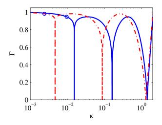
Figure 3: Comparison between optimal P = 3 scheme for N = 16 (· - ·)and N = 32 (-).  $\Gamma(\kappa_{\min})$  for each case is denoted by  $\circ$ . For the curve of N = 16,  $\kappa_{\min} = 0.0096$ ,  $\kappa_1 = 0.0351$ ,  $\kappa_2 = 0.4282$  and  $\Gamma_{\max} = 0.946$ , while for the N = 32 curve,  $\kappa_{\min} = 0.0024$ ,  $\kappa_1 = 0.0125$ ,  $\kappa_2 = 0.2689$  and  $\Gamma_{\max} = 0.981$ .
